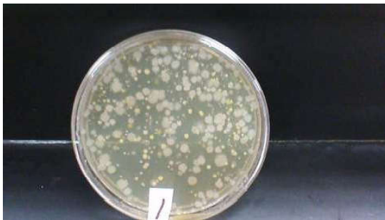
Figure 8A: Coliform Bacterial growth from collected water samples indicative of water pollution.
